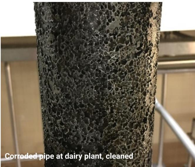
“See, Jim?” I pressed, “Not only is it brown and covered in corrosion, but as you can see in the second photo, after we cleaned the pipe, the pitting is so significant you can see it from a few feet away! You must admit, this needs to be replaced with new pipe.
